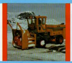
PV 210S/HH 750 Performance 750-1000 HP Capacity up to 12 tons/HPh Impeller diameter 2.1 m Clearing width 3.2 m Clearing height 2.4/3.0 m Weight 20.000 kg Max. speed 40 km/h
